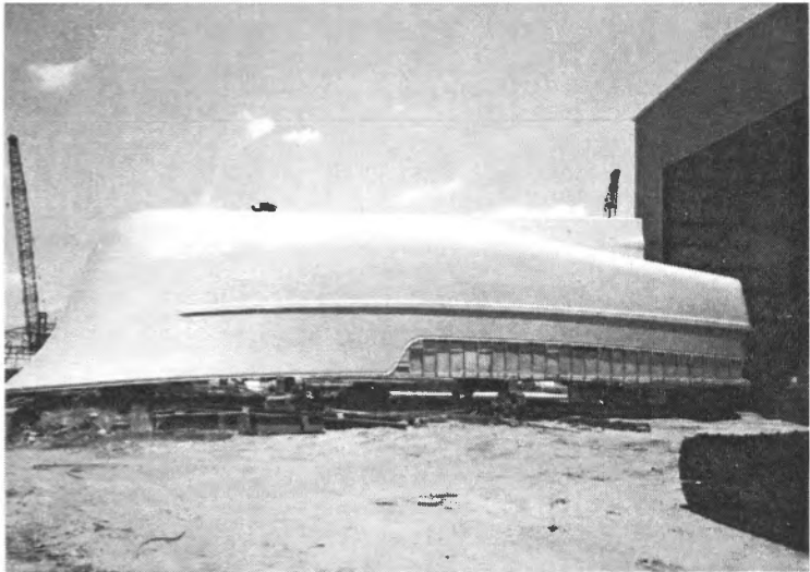
83ft. Boat emerging from its mould.
