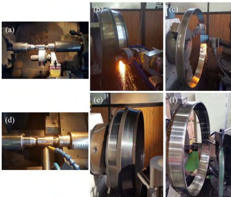
Fig. 1. Polishing and UNSM treatment process of (a, d) rollers, (b, e) inner ring, and (c, f) outer ring
