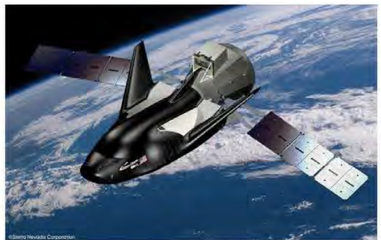
Space utility vehicle: Sierra Nevada's unmanned Dream Chaser is designed to haul 6 tons of cargo to and from the International Space Station. COURTESY COMPANY
